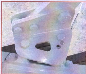
Working width to be changed mechanically. Three working width positions: 32 - 40 - 45 cms.
