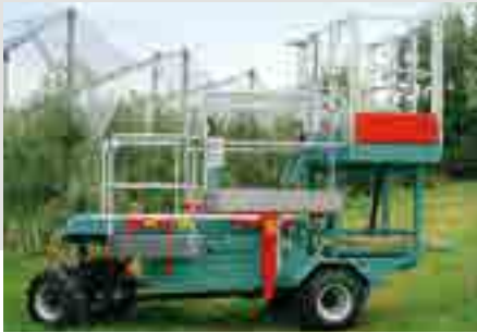
A special platform for the installation and maintenance of hail nets
