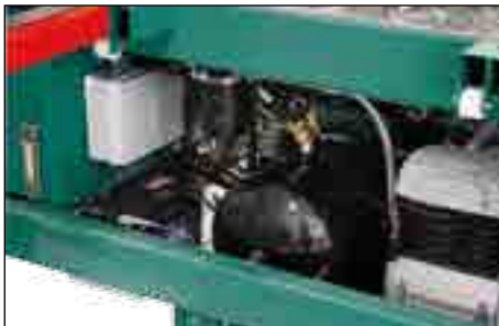
Air compressor 650lt inside the machine
